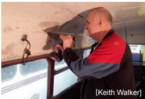
Jeff de-rivetting 243's internal roof trim.
